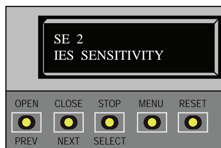
Figure 46. Adjusting IES Sensitivity
