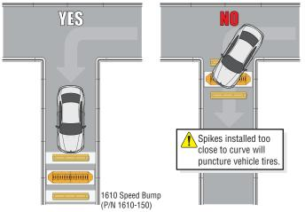
Traffic spikes must be installed on a flat-level concrete surface avoiding bumps or dips including uphill or downhill slopes minimizing the possibility of water draining into the spike assembly. Asphalt, brick, dirt, gravel or worn out concrete are not appropriate installation surfaces. If traffic spikes are needed in an area that has an inappropriate road surface, a leveled concrete pad must be laid out covering the entire spike area.
