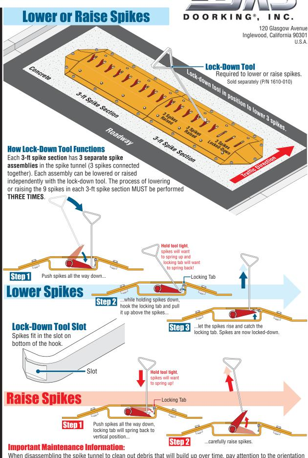
of the springs for the spikes and locking tabs. They MUST remain in the factory installed orientation or the spike
